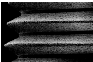
Figure 7 Stern EX Dental Implant SEM – Scanning Electron Microscopy
